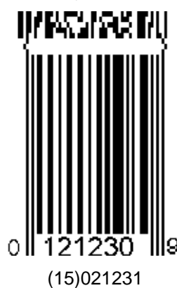
Figure 5.8.8 – 4. UPC-E Symbol with a Two-Column CC-A
