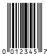
Figure 5.2.1.3.4 – 1. UPC-E Bar Code (Encoding 001234000057 by Zero-Suppression)
