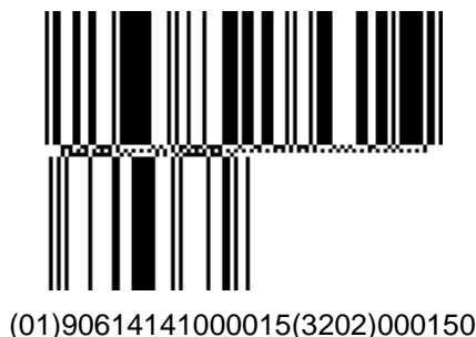
Figure 5.6.1.4.2 - 1. GS1 DataBar Expanded Stacked Bar Code
