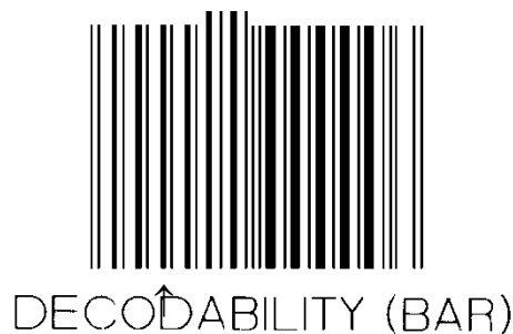
Figure 5.5.3.3.12 – 3. Calibration Symbol with Engineered Low Decodability Grade
