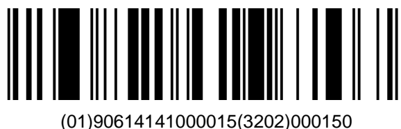
Figure 5.6.1.4.1 – 1. GS1 DataBar Expanded Bar Code
