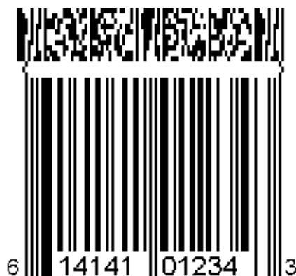
Figure 5.8.8 – 2. UPC-A Symbol with a Four-Column CC-B Component
