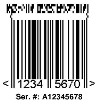
Figure 5.8.8 – 3. EAN-8 Symbol with a Three-Column CC-A
