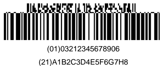
Figure 5.8.8 – 9. GS1-128 Symbol with a Four-Column CC-A
