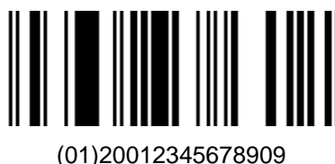
Figure 5.6.1.2.1 – 1. GS1 DataBar Omnidirectional Bar Code
