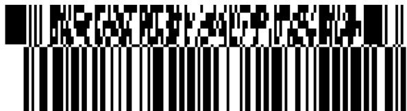
Figure 5.8.2 – 2. GS1-128 Composite Symbol with CC-C
