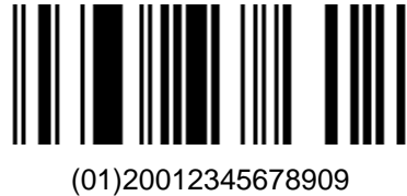
Figure 5.1 – 4. GS1 DataBar Omnidirectional Bar Code
