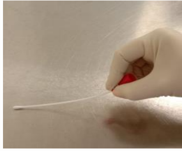
Figure 2. Swab positioning during sampling.
